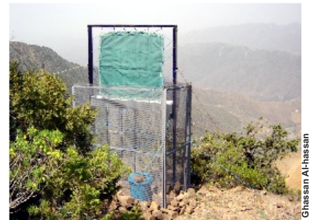
Initial fog collector, with protective fence, at 3200 m elevation in the southwest of Saudi Arabia.
