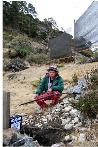
One of the data loggers installed by Rick Taylor in Guatemala to measure the amount of water produced by the fog collectors.
