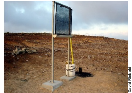
The collector to measure fog fluxes at Aganada, Lanzarote, Spain.
