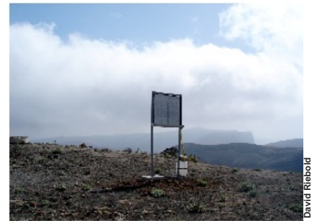
The collector to measure fog fluxes at La Quemada, Lanzarote, Spain.
