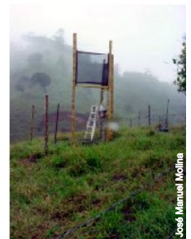
Two SFCs installed at right angles in Columbia.
